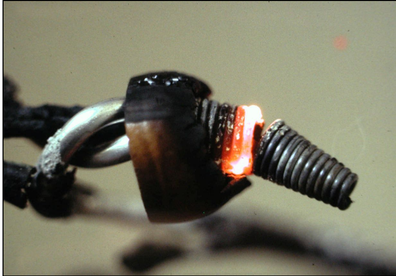
FIGURE 1 - ALUMINUM WIRE SPLICES MADE WITH TWIST-ON CONNECTORS CAN BE DANGEROUS. The use of most types of twist-on connectors with aluminum wire can lead to hazardous results. This twist-on pigtail connection (two #10 aluminum wires with one #12 copper wire, in a 20-amp circuit), made with a twist-on connector that was UL listed for use with aluminum wire at the time, remains electrically functional in the circuit, but it becomes extremely hot whenever a significant amount of current flows. The heat has deteriorated the insulation on both the connector and the wires. In this photo, a portion of the connector's spring is red hot, at current well below the circuit rating.
